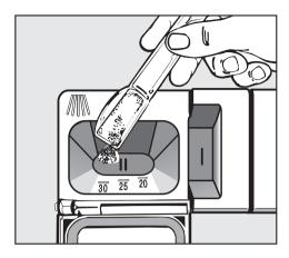
The horizontal marks in Compartment II indicate levels of approximately 1 <sup>1</sup>/<sub>4</sub>, 1 <sup>3</sup>/<sub>4</sub> and 2 tablespoons (20, 25 and 30 ml) respectively.
